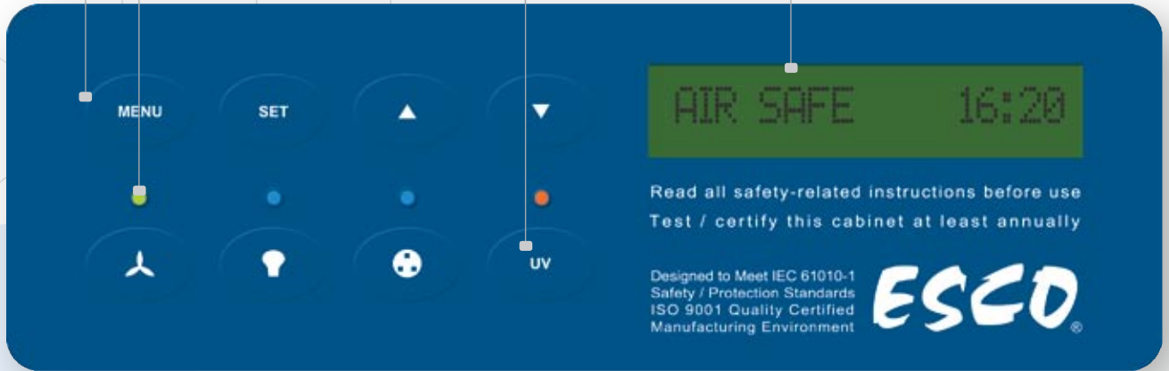
Sentinel Microprocessor Control System, Programmable
